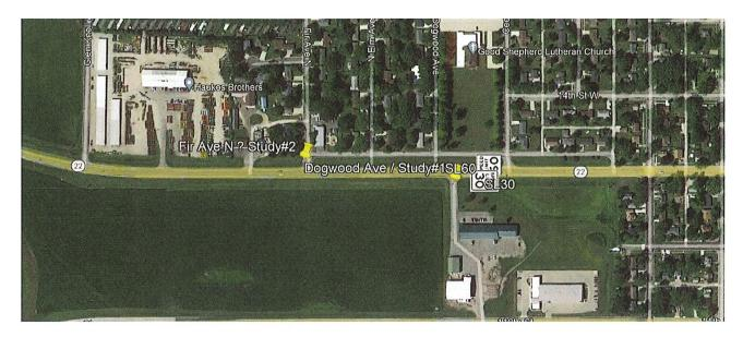
Note, a public road connection south of Fir Ave is proposed. The connection will provide access to future development south of TH 22. The existing bypass south of Fir Ave will be removed and a right turn lane will be constructed.
